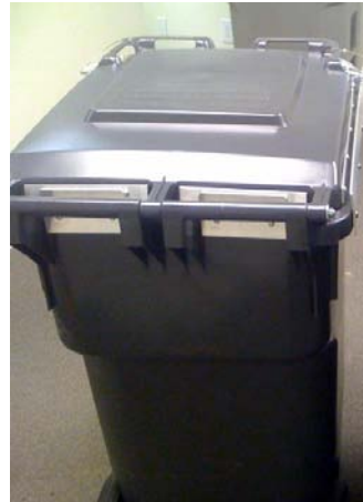
Growler Can with Metal Plate Reinforcements As Tested
